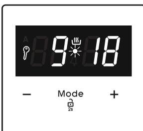
After a few seconds, the dot will stop flashing and will remain illuminated.
