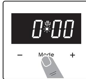
To unlock the timer buttons, press and hold the "MODE" button for 2 seconds. The desired operation can then be carried out.
